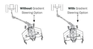
In this illustration the front wheels are free to caster and the mower is skewed noticeably.
