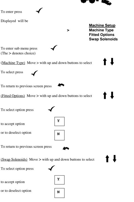
With this facility it allows operations of functions to be swapped without changing the wiring or hoses
