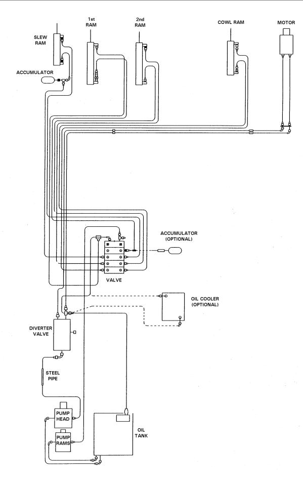
HOSE CIRCUIT DIAGRAM (Power Slew Machines) 16-8
