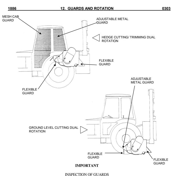
Inspect guards twice daily or immediately damage is suspected.
