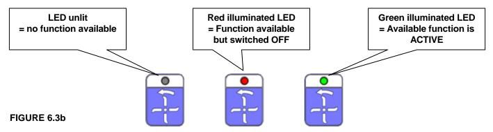
Each button is accompanied by a bi-colour LED. When the control box is connected and powered up all available services are illuminated in red. LED's which remain 'off' indicate services which are not available on the machine. When a red illuminated (available) LED service is subsequently activated the LED changes colour from red to green.
