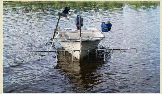
The Dorocutter Klippo is a machine in the middle class. All maneuvering of Klippo is done from the drivers seat, like deep-going and the drift of the knife. The knife can be angled for cutting in blanket of plants and cutting close to land. Klippo is equipped with rockreleasing and has an adjustable frame for diffrent boatwidths.
