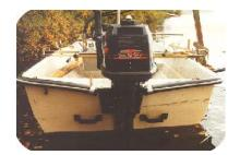
Sidemounted reedcutters pull the boat sideways. This is compensated if the boatengine is mounted a little bit to the right.
