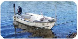
The Dorocutters can be used effectivly with the Reed rake. The reed that sometimes disturb the propeller is steered away with the rake. The rake is used together with Hymo, Klippo, Wasse och Elis.
