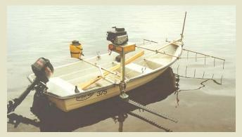
The Dorocutter Wasse is our smallest engine powered reedcutter. Wasse is the suitable reedcutter when small areas and diffrent watersystems are maintained. The cutting deep, the drift of the knife, start and stop of the engine etc. are done from the drivers seat. The ligth construction makes transport and mounting easy. Rockreleaser is standard.
